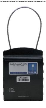
RadioSecure™ SLG-d is the latest innovation in the RadioSecure™ family. It meets the industry's needs for a low cost yet reliable device to accurately tracks intermodal containers and conveyances using active RFID, GPRS, GPS and Satellite Communication technologies.
